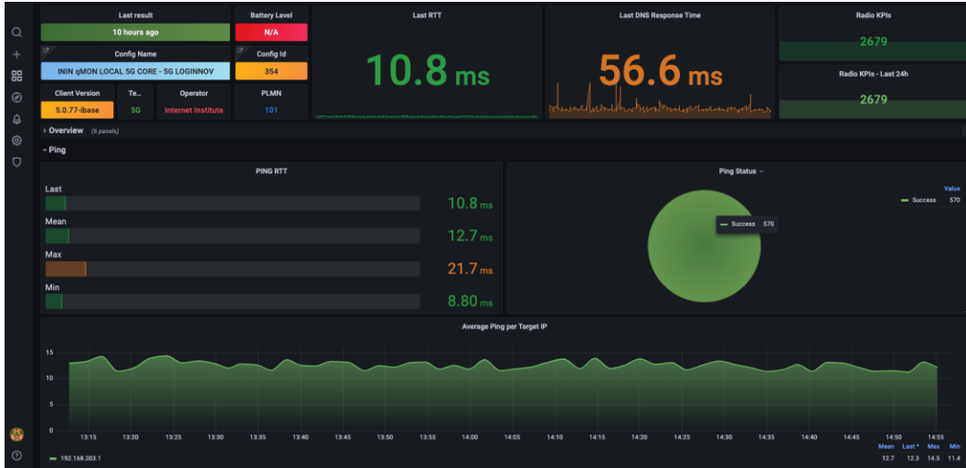
Figure 7: KPI results visualization collected as part of a 5G network continuous monitoring.
